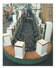
Most manufacturers' evacuation realization consists of a moving production line or carousel where each refrigeration circuit or other product is attached to a single smaller rotary pump (10-20 m³/h). This method eliminates every one of the disadvantages of the manifold system while adding additional benefits.
